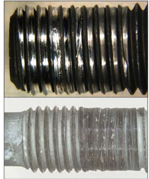
Damaged thread on actuator
