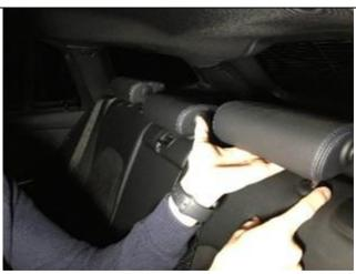
a. If the headrest cannot be lifted out of the seat, the positive stop is present.
