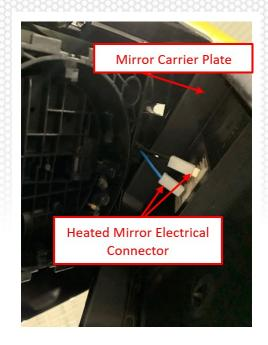
**3.** Using the new replacement mirror carrier plate, position the heated grid so it is in the upper position and then connect the two electrical connectors to the heated grid.
