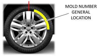
Inspect DOT number and mold number on all four tires and replace affected tires if necessary.
