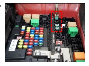
3. Install the new required two (2) new 30A fuses.
