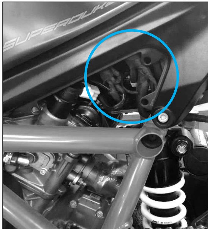
Fig. 10 - Main wiring harness area to be checked
