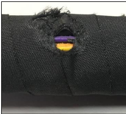
Fig. 4 - Mild or no Damage (follow code 00)
