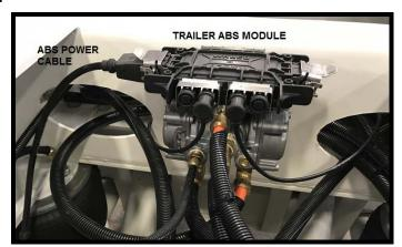
Figure 1 ABS Module and ABS Power Cable
