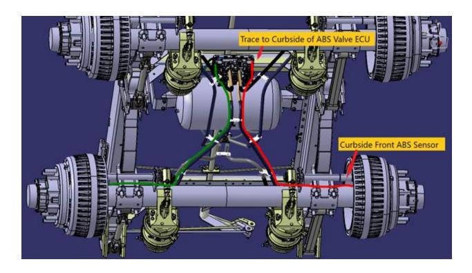
The view below shows what it would like if the sensor cables are installed incorrectly. The sensor cables should not cross side to side.
