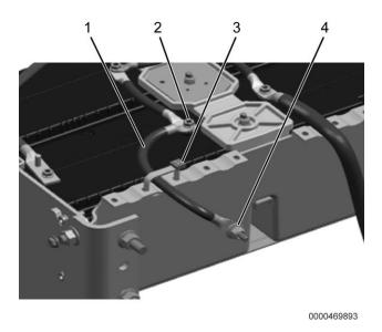
Figure 1. Routing of New Battery Cable for Population 1
