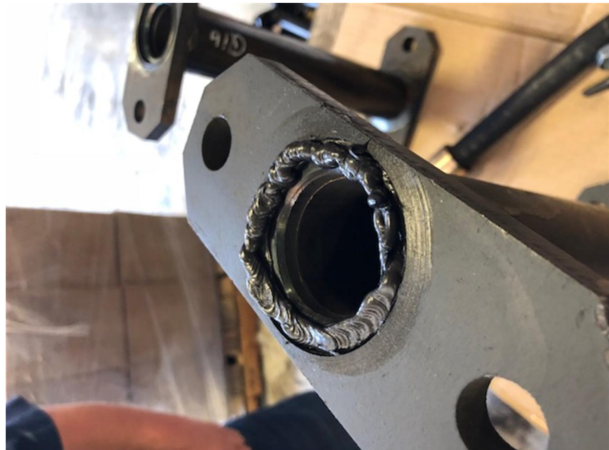
^ STEP 1: 1/4" BEAD IN STEP (CALIPER SIDE)
