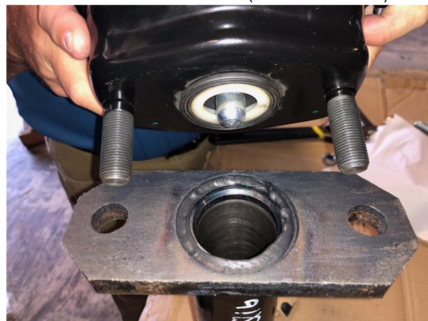
v STEP 1: 1/8" BEAD IN STEP (CHAMBER SIDE)
