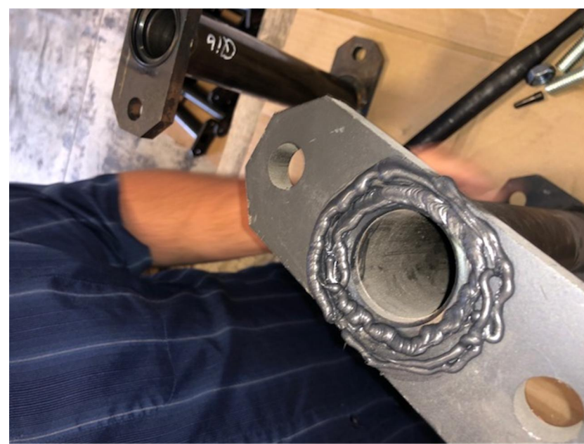
^ STEP 2: 1/8" BEAD AROUND HOLE (CALIPER SIDE)
