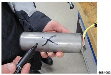
6. Put a mark on the removed inflator and store it in the replacement part box.
