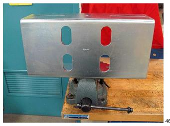
1. Mount the airbag module bracket securely in a vise.
