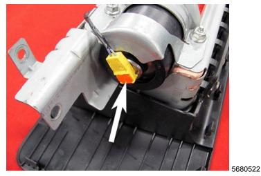
27. Install the black taped wire into the inflator (black cap end). Ensure the CPA is engaged.
