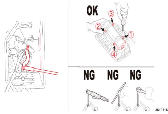
23. Tighten four (4) *NEW* plate nuts evenly in several increments in the order shown in the illustration using a 10-mm socket driver while pushing on the inflator against the alignment tab.
