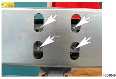
3. Position the airbag assembly so that all four stopper plate nuts can be removed through the access holes.
