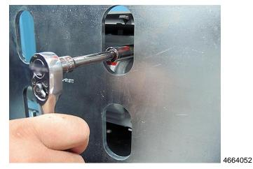
8. Use the access holes in the bracket to loosen and remove the four self-locking nuts, **do not use power tools to remove the nuts**. Discard the nuts, they will not be reused.
