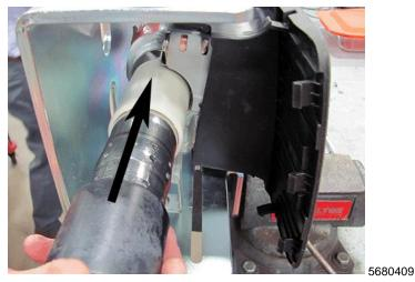
11. Carefully slide the new inflator into the airbag assembly. Ensure the inflator is installed with the harness (white end cap) end first.
