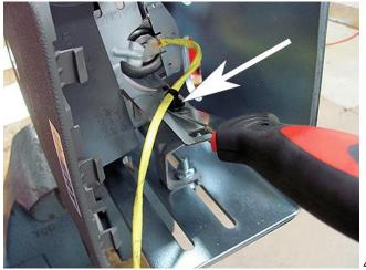
3. Disengage the wire harness locator from the housing.
