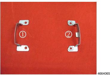
2. Remove the two stopper plates (1 and 2). Discard the stopper plates, they will not be reused.
