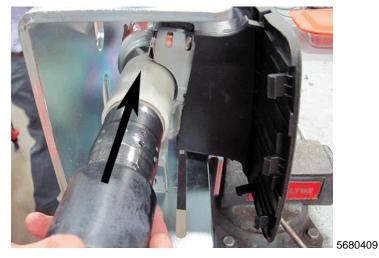
19. Slide the new inflator into the housing with the white end cap first.
