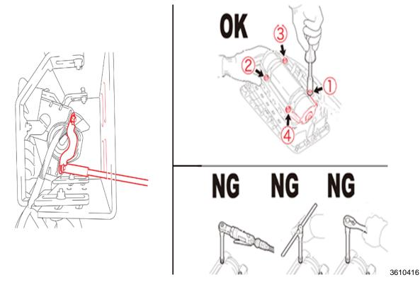
15. Tighten four (4) *NEW* plate nuts evenly in several increments in the order shown in the illustration using a 10-mm socket driver while pushing the inflator. You will encounter some resistance during tightening because these nuts are self-locking nuts. **Torque Specification: 6.5 Nm (57 in-lb).**
