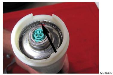
• Ensure the tab on the white end cap is aligned with the notch in the inflator.
