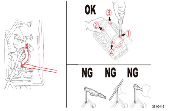
22. Tighten four (4) *NEW* plate nuts evenly in several increments in the order shown in the illustration using a 10-mm socket driver while pushing on the inflator against the alignment tab.
