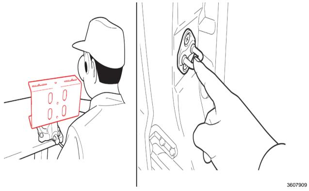
**Danger:** To avoid personal injury, *ALWAYS* keep as much of your body as possible in front of the bracket when working on the airbag assembly. Remember to periodically touch a metallic part of the vehicle or work bench to discharge static electricity in the body. DO NOT use power tools when performing the inflator removal/reinstallation steps.
