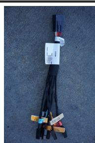
**Step 15:** Plug the rework harness into terminal P04B Spare batt 1
