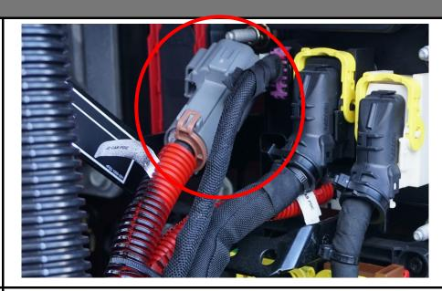
**Step 2:** Remove Lower panels on LH side (5 screws) (2 connectors)
