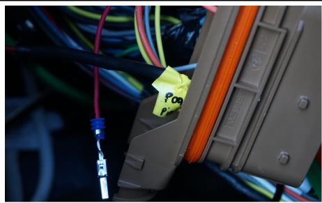
**Step 13:** Replace pin 17 in connector P006 (gray) with RED 0731-10 on the rework harness:
