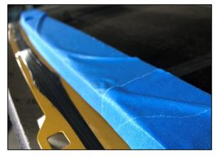
Apply collision wrap or window guard wrap to prevent debris from entering the interior of the vehicle.
