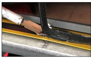
5. Use the scraper tool to cut through the urethane while continiously peeling it away.
