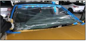
With a razor blade or a urethane scraper, make a cut through the urethane (rubber sealant) on the flange.
