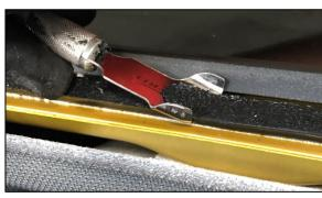
4. Pry up a side of the urethane and peel it away from the flange.
