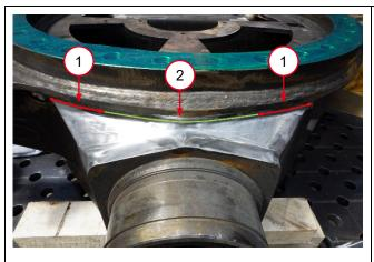
Remove the paint before evaluating a crack for its priority. A crack is in the critical zone if it reaches into the critical area (1) in either the right or the left side.
