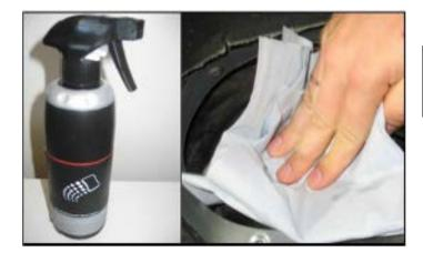
Clean top of fuel filter with suitable plastic cleaner.
