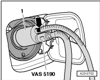
If fuel was removed due to replacement of the fuel filter flange, dispense recovered fuel contained in the -VAS 5190- Fuel Extracting Device back into the vehicle fuel tank at this time.
