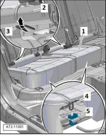
Remove right rear cushion <2> by lifting upwards and pulling outward to remove the seat cushion.
