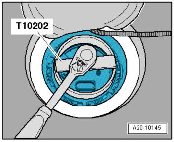
Reinstall the fuel filter flange locking ring by turning clockwise. Torque the locking flange to 110 Nm.
