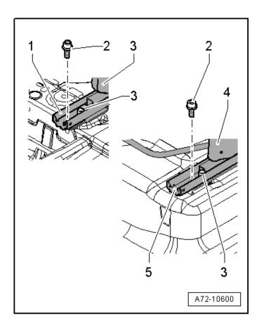
Remove the seat rail stop bolts <2> (if required).
