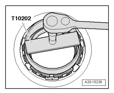
Tighten the locking ring using the Fuel Sending Unit Wrench -T10202-. Torque the locking flange to 110 Nm.
