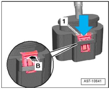
Be sure to properly engage the red locking tab <1> by pressing down <arrow> after properly securing the connector.
