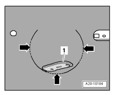
If necessary, cut the floor covering along the perforation <arrows> on the left side with a carpet knife <1>.
