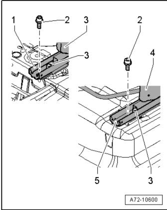
• Reinstall the seat rail stop bolts <2>. Tighten the bolts to 20 Nm.
