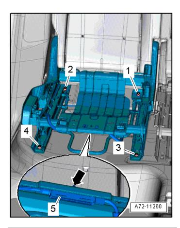
• Remove the four right rear seat frame bolts <1, 2, 3, and 4> using hand tools.
