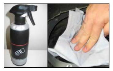
Clean top of fuel pump with suitable plastic cleaner.
