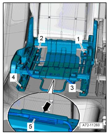
• Remove the right rear seat frame assembly from the vehicle.
