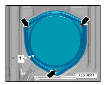
Remove the fuel pump flange cover <1> by removing the three screws <arrows>.
