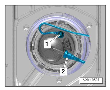
Remove the fuel line connector <2> from the locking flange by squeezing the release tab between the finger and thumb, pushing in on the connector, and then pulling the connector off.
