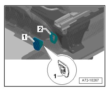
Reinstall seat rail cover trim <1> onto seat frame <2>.
