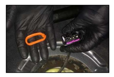
If required, repair the wiring harness connector, wiring, and weather pack seals before reconnecting the connector to the fuel filter flange.
