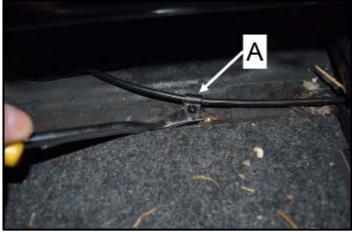
For vehicles equipped with adjustable seat frames, slide the seat frame forward and unclip the seat frame adjustment cable from the threaded tab <A>.
