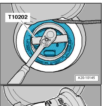
Using Fuel Sending Unit wrench -T10202-, remove the locking ring from the fuel pump flange by turning counterclockwise.
