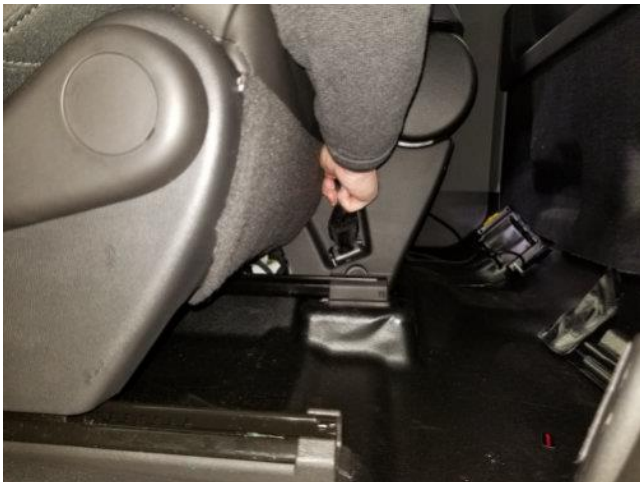
Seat-Belt Bracket Positioned Too High, Securing Bolt Not Through Hole in Bracket.
