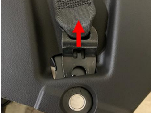
Seat-Belt Bracket Positioned Too High, Securing Bolt Not Through Hole in Bracket.
