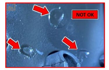
• Inspect the underside of the footpad on the brake pedal using an inspection mirror.
