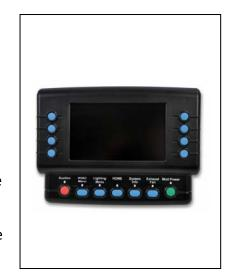
when starting the engine, the V-MUX® Vista IV Interface typically turns off and quickly and automatically restarts. However, units on the attached list may not restart on their own if the voltage dips out of range (less than 9 volts).
