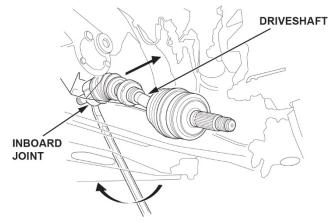
7. Drive the inboard joint off of the intermediate shaft using a drift punch and a hammer. Remove the driveshaft as an assembly.
