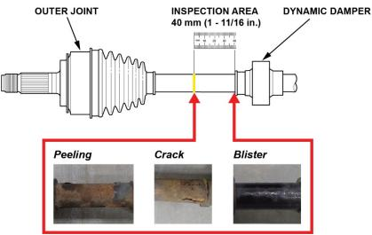
Is there peeling paint, cracks, or blisters on the driveshaft within 40 mm (1-11/16in) of the dynamic damper?
