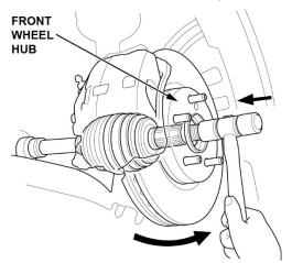
Left driveshaft: Pry the inboard joint using a pry bar. Remove the driveshaft as an assembly.
