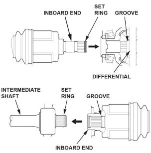
13. Make sure the connecting surfaces of the joint and splined section are clean of any debris or rust particles using a shop towel and/or compressed air before starting installation. Apply about 5 g (0.18 oz) M-77 Assembly Paste (P/N 08798-9010) to the contact area of the outboard joint and the front wheel bearing.
