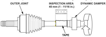
Using the masking tape as a guide, trace a line all around the axle using the yellow paint marker.
