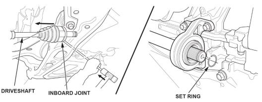
Insert the inboard end of the driveshaft into the differential until the set ring locks in the groove.
