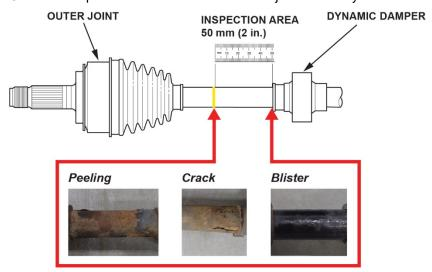
Is there peeling paint, cracks, or blisters on the driveshaft with 50 mm (2 in) of the dynamic damper?
