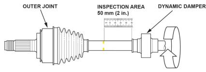
5. Connect the 4 painted dots around the axle using masking tape.
