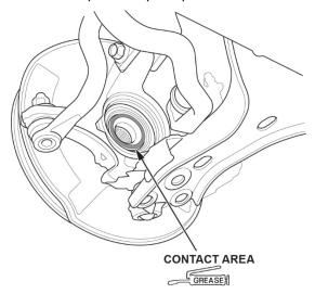
13. Install the outboard joint into the front wheel hub.
