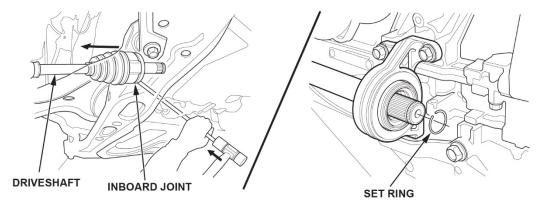
10. Left Driveshaft: Clean the areas where the driveshaft contacts the differential thoroughly with solvent. Dry the areas where the driveshaft contacts the differential thoroughly with compressed air
