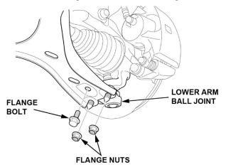
5. Pull the knuckle outward and separate the outboard joint from the front wheel hub using a plastic hammer.
