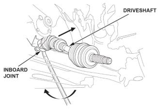
8. Drive the inboard joint off of the intermediate shaft using a drift punch and a hammer. Remove the driveshaft as an assembly.
