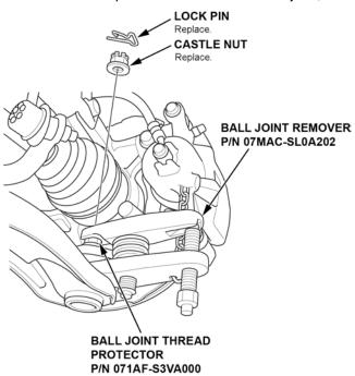
4. Separate the ball joint from the knuckle using the Ball Joint Thread Protector (T/N: 07AAF-SDAA100) and Ball Joint Remover (T/N: 07MAC-SL0A202). Grease the threads and tip of the pressure bolt on the ball joint remover, and make sure the pivot bolt is not parallel to the ball joint remover arms. For additional information on how to use the tools, refer to the service information.
