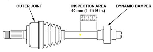
4. Rotate the axle 1/4 turn and repeat the step above three times until there are four paint dots on the axle.
