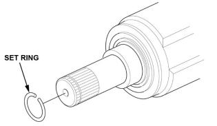
10. Passenger's side driveshaft only: Replace the set ring on the intermediate shaft.
