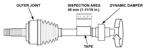
6. Using the masking tape as a guide, trace a line all around the axle using the yellow paint marker. Marking the line accurately is important, especially if there is damage close to or inside the 40 mm line.
