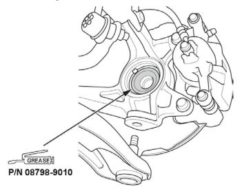
13. Insert the inboard end of the driveshaft into the differential or intermediate shaft until the set ring locks in the groove. Make sure to insert the driveshaft(s) straight in to avoid damaging the oil seal.
