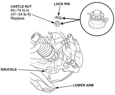
16. Install the new castle nut, and torque it to the lower torque specification. Then, tighten it until the slot on the castle nut aligns with the ball joint pin hole. Install the lock pin into the pin hole as shown.
