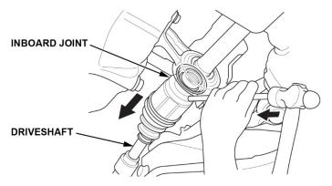
9. Driver's side driveshaft only: Replace the set ring on the inboard joint.
