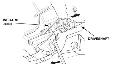
8. *Passenger's side driveshaft only*: Using a punch and hammer, drive the inboard joint off of the intermediate shaft. Then, remove the driveshaft as an assembly.
