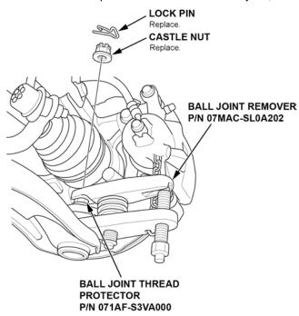
4. Separate the ball joint from the knuckle using the Ball Joint Thread Protector (T/N: 071AF-S3VA000) and Ball Joint Remover (T/N: 07MAC-SL0A202). Grease the threads and tip of the pressure bolt on the ball joint remover, and make sure the pivot bolt is not parallel to the ball joint remover arms. For additional information on how to use the tools, refer to the service information.
