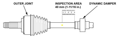
4. Rotate the axle 1/4 turn and repeat the step above three times until there are four paint dots on the axle.
