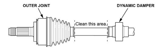
3. Using a ruler and yellow paint marker, measure **40 mm (1-11/16 in)** away from the dynamic damper, and mark the driveshaft with a dot. Click <u>HERE</u> to view a video on how to do the inspection procedure.
