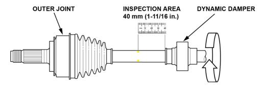
5. Connect the four painted dots around the axle using masking tape.
