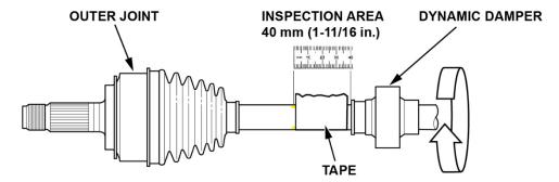
6. Using the masking tape as a guide, trace a line all around the axle using the yellow paint marker. Marking the line accurately is important, especially if there is damage close to or inside the 40 mm line.
