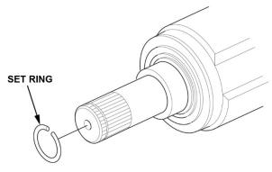
10. Passenger's side driveshaft only: Replace the set ring on the intermediate shaft.
