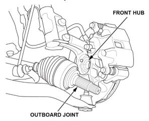
15. Wipe off any grease contamination from the tapered ball joint section and threads, then install the knuckle onto the lower arm. Make sure not to damage the ball joint boot.
