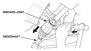
9. Driver's side driveshaft only: Replace the set ring on the inboard joint.
