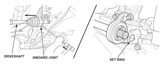
9. Insert the inboard end of the driveshaft into the differential until the set ring locks in the groove.
