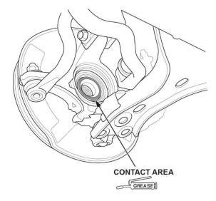
14. Install the outboard joint into the front wheel hub.
