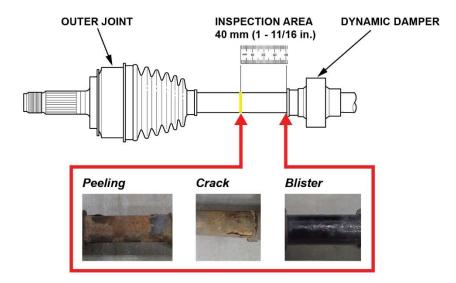
Is there peeling paint, cracks, or blisters on the driveshaft within 40 mm (1-11/16in) of the dynamic damper?
