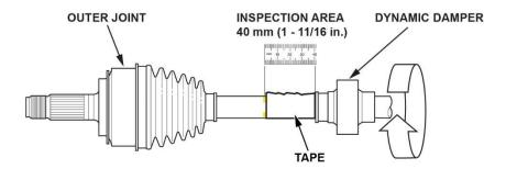
6. Using the masking tape as a guide, trace a line all around the axle using the yellow paint marker.
