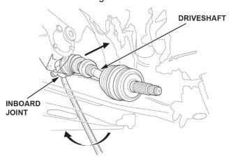
7. Drive the inboard joint off of the intermediate shaft using a drift punch and a hammer. Remove the driveshaft as an assembly.
