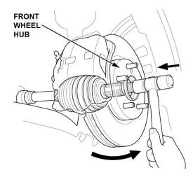
6. Left driveshaft: Pry the inboard joint using a pry bar. Remove the driveshaft as an assembly.
