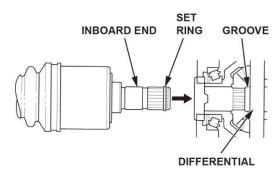
10. Left driveshaft: Clean the areas where the driveshaft contacts the differential thoroughly with solvent.
