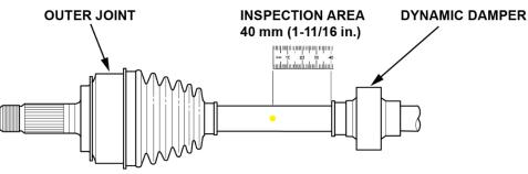
4. Rotate the axle 1/4 turn and repeat the above step 3 times until there are 4 paint dots on the axle.
