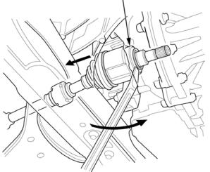
6. Remove the left driveshaft as an assembly.
