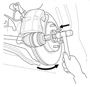
5. Use a pry bar to pry the inboard joint of the left driveshaft from the transmission.
