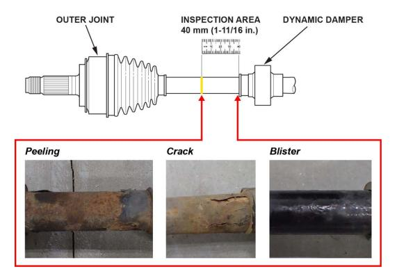
NOTE: Corrosion or paint defects between the outer joint and the yellow line are OK.
