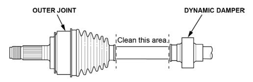
3. Using a ruler and yellow paint marker, measure **40 mm (1-11/16 in)** away from the dynamic damper, and mark the driveshaft with a dot. Click <u>HERE</u> to view the video on how to do the inspection procedure.
