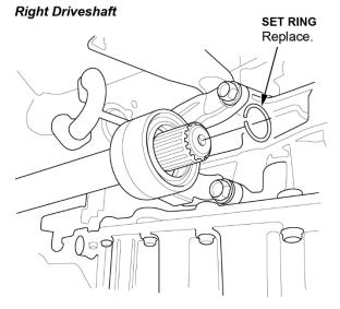
10. Make sure the mating surfaces are clean, then install the new driveshafts. Insert them until the set rings lock in the grooves.
