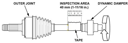
6. Using the masking tape as a guide, trace a line all around the axle using the yellow paint marker.
