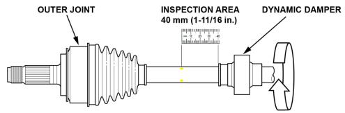
5. Connect the 4 painted dots around the axle using masking tape.
