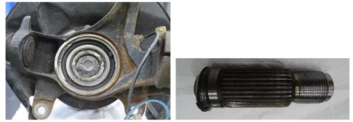
15. Use a drift punch to stake the spindle nut shoulder against the notch on each driveshaft.
