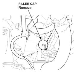
22. Fill the transmission with a suitable amount of HCF-2 CVT Fluid.
