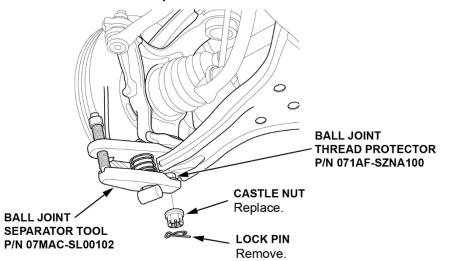
4. Use a soft-face hammer to separate the outboard joints from the steering knuckles.
