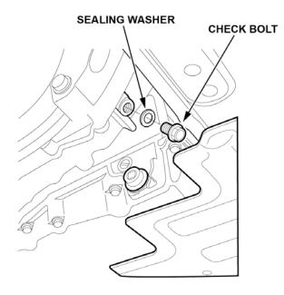
The transmission is at the proper level if the fluid is dripping from the hole gradually.
