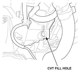
23. Install the filler cap in the direction shown and restart the procedure at step 17.
