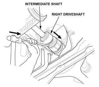
8. Remove the right driveshaft as an assembly.
