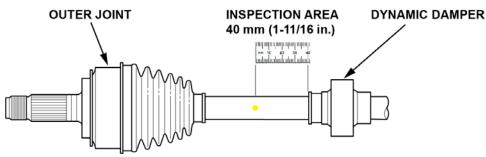
4. Rotate the axle 1/4 turn and repeat the above step **3 times** until there are 4 paint dots on the axle.
