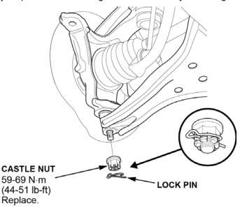
14. Install the new spindle nuts provided in the hardware kit.
