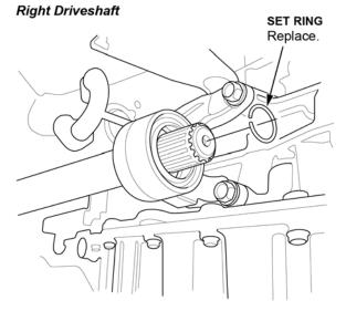
10. Install the new driveshafts. Insert them until the set rings lock in the grooves.
