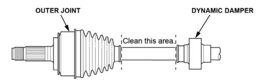
3. Using a ruler and yellow paint marker, measure **40 mm (1-11/16 in)** away from the dynamic damper, and mark the driveshaft with a dot. Click <u>HERE</u> to view the video on how to do the inspection procedure.
