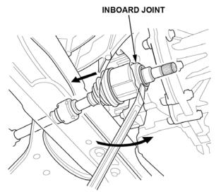
6. Remove the left driveshaft as an assembly.
