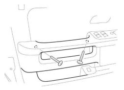
6. Carefully pry out the mirror mount cover by hand in the sequence shown.
