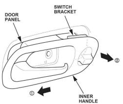
4. Disconnect the power door lock switch connector. Disconnect the inner handle rod, and remove the inner handle.
