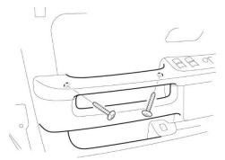
6. Carefully pry out the mirror mount cover by hand in the sequence shown.
