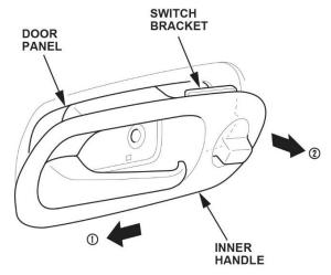
Disconnect the power door lock switch connector. Disconnect the inner handle rod, and remove the inner handle.
