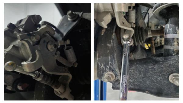
(3) Replace the Caliper Body Assembly
