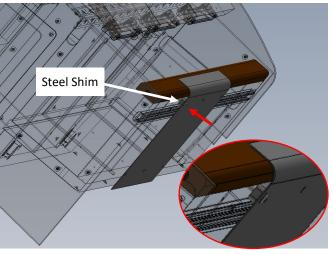
Line up the tip of the screw with the mark so the curve of the heat shield is firmly up against the curved edge of the face of the cabinet. Drive screw into base of overhead cabinet approximately half
