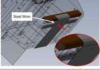
1. Secure the center screws into the cabinet.
