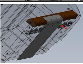
Secure front plate and shim to cabinet base approximately half way.
