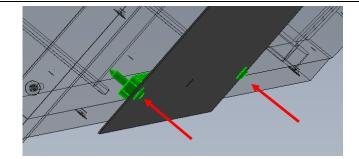
Slip the rear shim between the heat shield and the cabinet and secure with a screw on each end.
