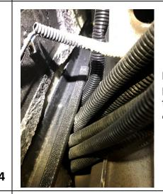
If no damage is found, install the 200mm piece of split tubing (126-6603) over top of the Sprinter harness at the potential contact point with the tank bracket.
