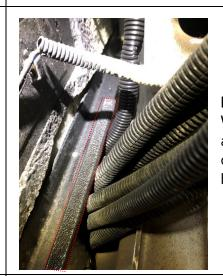
Install a 200mm (8 inches) piece of Windlace (140-3021) on the side of the angled hanger bracket at the potential contact point to protect the wiring harnesses.
