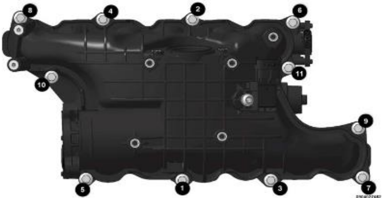
Figure 23 – Intake Bolts Tightening Sequence
