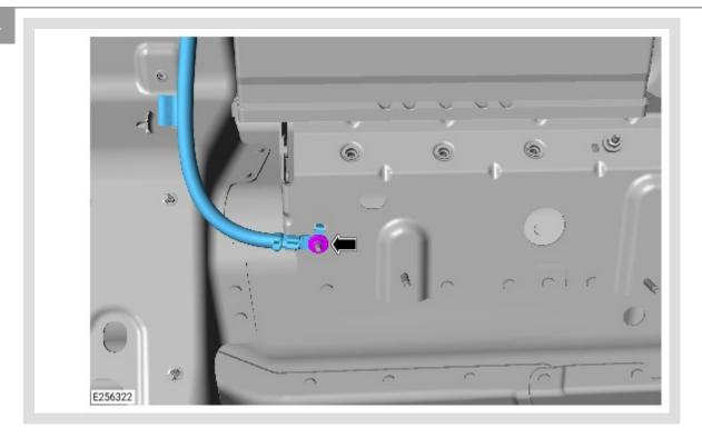
Remove the startup battery ground cable from the body ground stud (G4D178).
