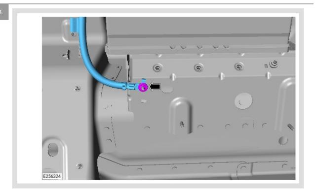
Install the startup battery ground cable to the new body ground stud.
