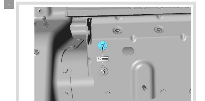
Install a new body ground stud (LR149837) 50 mm above the existing ground stud (see TOPIx Workshop Manual section 501-25A: Body Repairs General Information - General Procedures - Body Earth Stud Repair).
