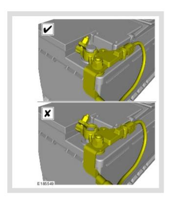
Connect the startup battery ground cable (see TOPIx Workshop Manual section 414-00: Battery and Charging System - General Information - Specifications).
