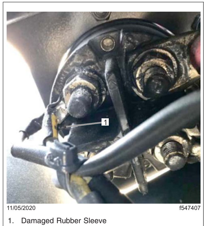
Fig. 3, Damaged Rubber Sleeve at the Back of the Battery Disconnect Switch
