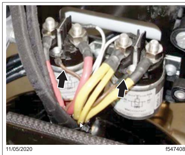
Fig. 7, Correct Installation Before Wax is Applied (relays shown)
