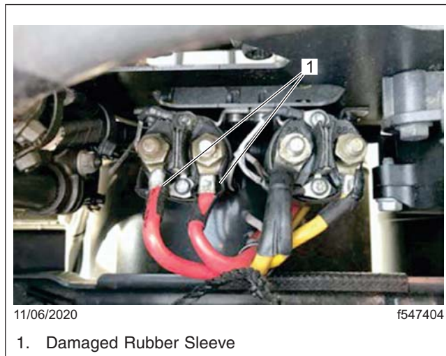
Fig. 2, Damaged Sleeve at the Relays
