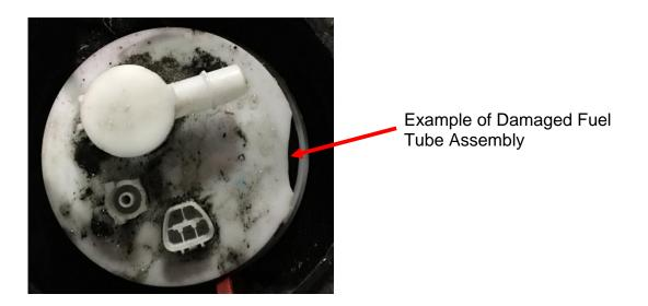
The damage during disassembly is caused by adhesion, or "sticking", of the Retainer Ring and the Fuel Tube Assembly. When the Retainer Ring is rotated on the stationary Fuel Tube assembly, the portions that are "stuck" together are under a very high load and may break off.
