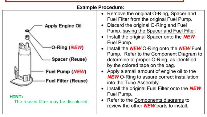
• Apply engine oil to the *NEW* O-ring before assembly to assure correct installation into the Fuel Suction Tube.
