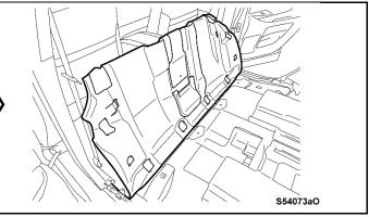
d. Remove the rear floor silencer pad No.2.
