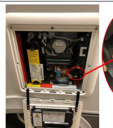
Open the Truma Water Heater door to access the Water heater 1/2" Female flare x 3/8" MPT connector to be replaced with a 3/8" Female flare x 1/2" Male flare coupling.
