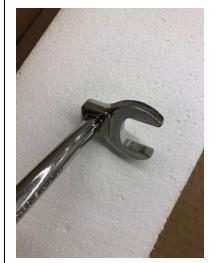
A 15/16" Open End Crowfoot Wrench can also be used if necessary to loosen the 3/4" flare nut.
