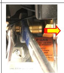
Push the pipe and nut to the right. Make sure there is ample propane line to push and the line does not kink. Check inside coach lines as well.
