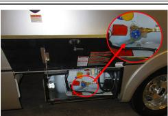
Turn off the Propane for the coach at the Solenoid (if equipped), or at the manual tank valve.
