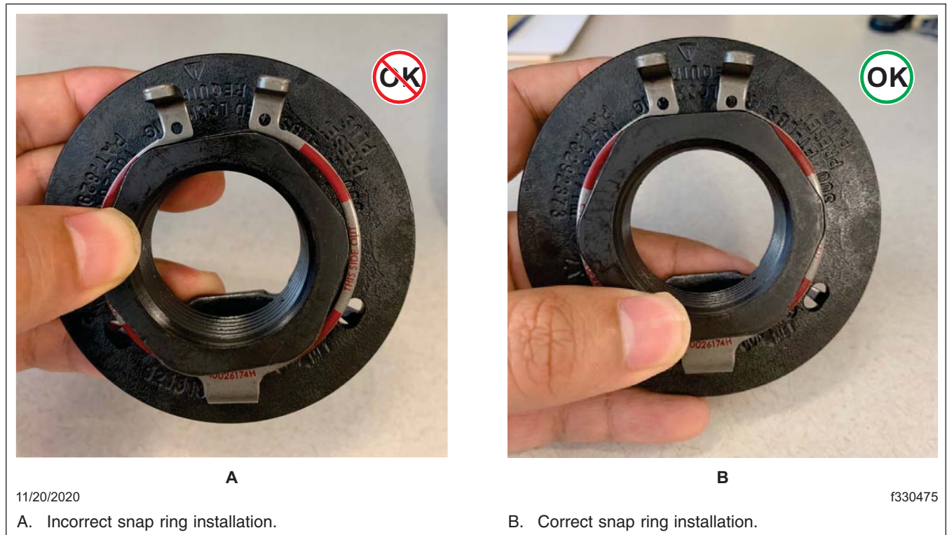
Fig. 3, Incorrect and Correct Snap Ring Installation Examples
