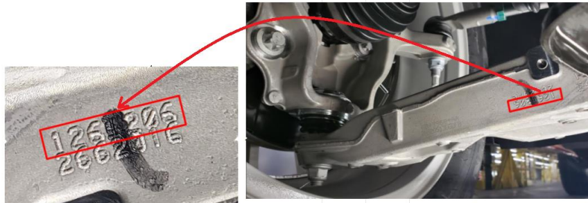
Figure 1 – Lower Control Arm Lot Number Inspection
