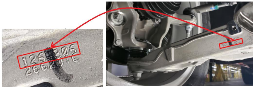
Figure 1 – Lower Control Arm Lot Number Inspection
