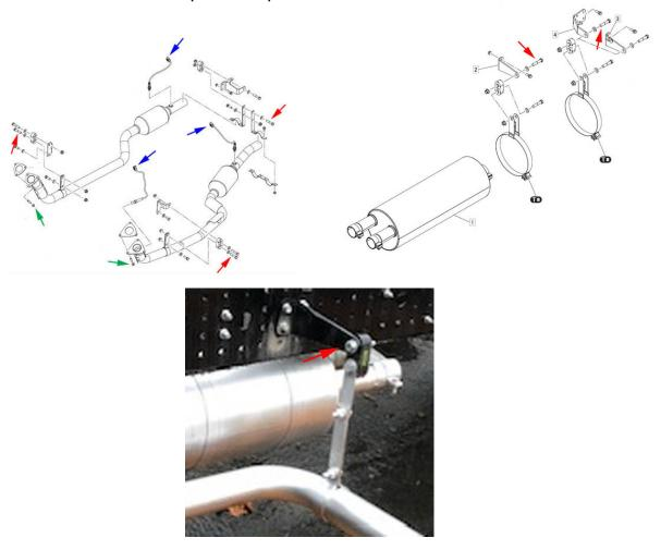
2. Remove the front exhaust pipes from the exhaust manifold flanges by lowering the complete exhaust system down as shown in the photo below left. Remove the gaskets from the studs as shown in the photo below right.
