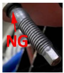
\*If any of the studs or nuts cannot be reused due to damage, replace them with OEM studs (ML296164) and nuts (ML296165).
