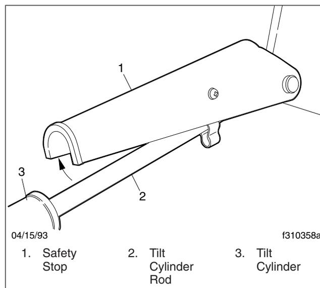
Fig. 24, Safety Stop Disengaged
