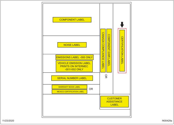
Fig. 6, FMVSS Certification Label Location, Recall Kit, Freightliner
