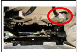
d. Disconnect the seat heater connection (if equipped)
