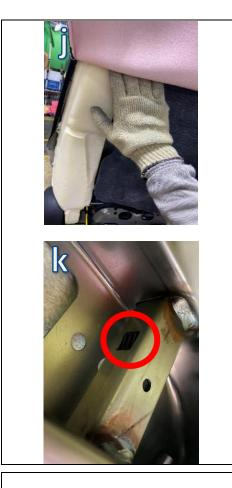
j. Lift back of seatback cover up to reach the headrest posts.
