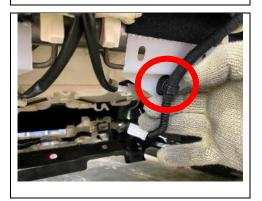
e. Unclip the seat heater wire harness from the seat frame (if equipped)
