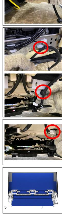
i. Pull the lower skirt tight to remove any wrinkles in the lower portion of the seatback cover
