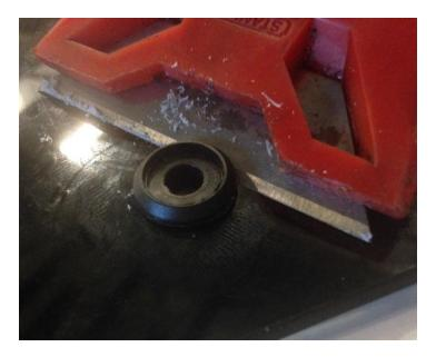
Remove the old glue from the mounting holes.
