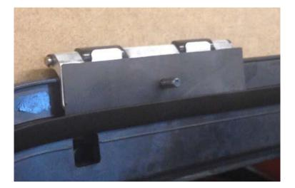
9. Install "E" clips onto the hinge pins.
