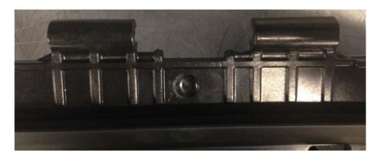
3. Use a putty knife to de-bond the plastic hinge strip from the glass. **Note:** Be careful when removing the plastic hinge strip not to scratch the surface.
