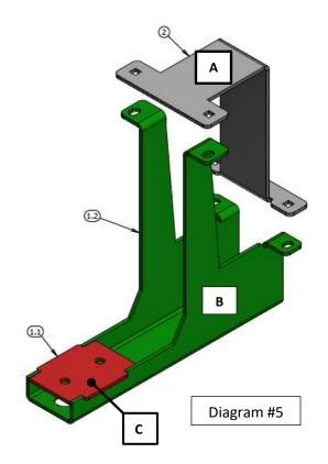
6. Set the hydraulic pump onto the top surface of the new bracket. (Picture #6) Insert the (2) new Hex Bolts through the top of the pump bracket (where the original bolts were). Set the hydraulic pump on the bracket, making sure the bolts are through the holes on the bracket plate C shown on Diagram #5. Adjust the hydraulic pump position as needed to insure it is securely seated on the bracket.
