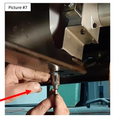
8. Using the long socket and ratchet, tighten the nuts through the holes in the bottom of the bracket. You may need to use the 9/16" open wrench to hold the bolt head while tightening the nut. Securely tighten nuts on both bolts. (Picture 8 & 9)
