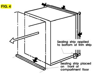
**NOTE**: Be careful not to damage the sealing strip applied to the floor of the enclosure when the refrigerator is put in place.
