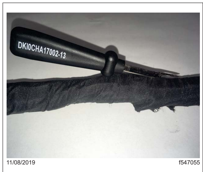
Fig. 5, Cutting the Fiber Wrap Using the Blunt End of the Seam Ripper
