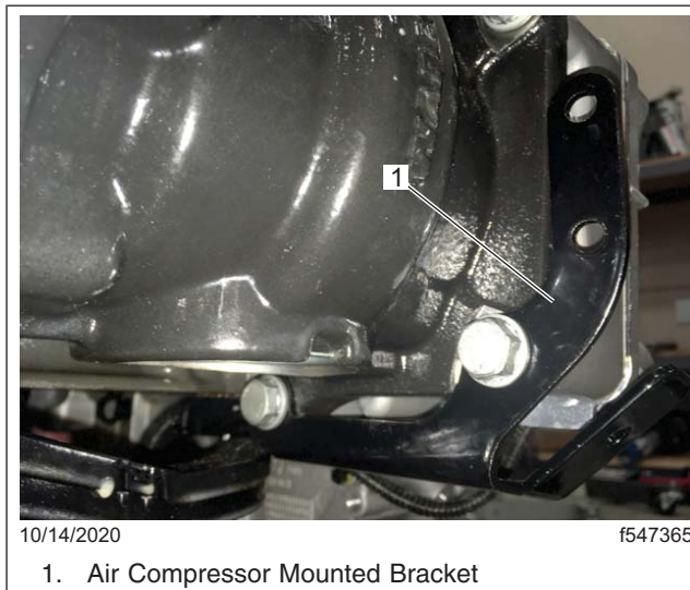
Fig. 15, New Air Compressor Mounted Bracket, Front View
