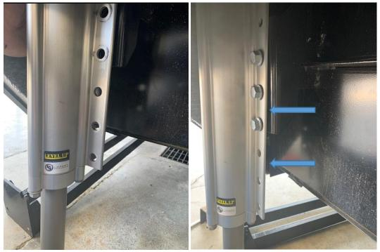
14. Lift bracket using floor jack into position between the front leveling jacks until the bottom set of holes on the bracket are lined up with the bottom set of holes on the jack leg.
